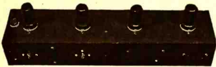
Top and bottom views of frequency-modulated transmitter. Coils are efficiently placed to keep oscillator and multiplier leads short.
